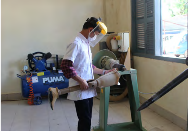
Bench Technician at Center for Medical Rehabilitation grinding a lower limb prosthetic device.
